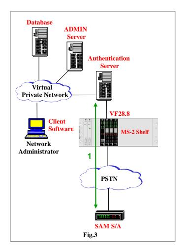
Fig. 3 shows the first secure dial-up call. The SAM generates a symmetric key that will be used to set up an AES tunnel. Both the symmetric key and the SAM ID are sent to the authentication server through an RSA encrypted tunnel. If the SAM ID is successfully authenticated, an AES tunnel is established and the authentication server sends the SAM a private key.
